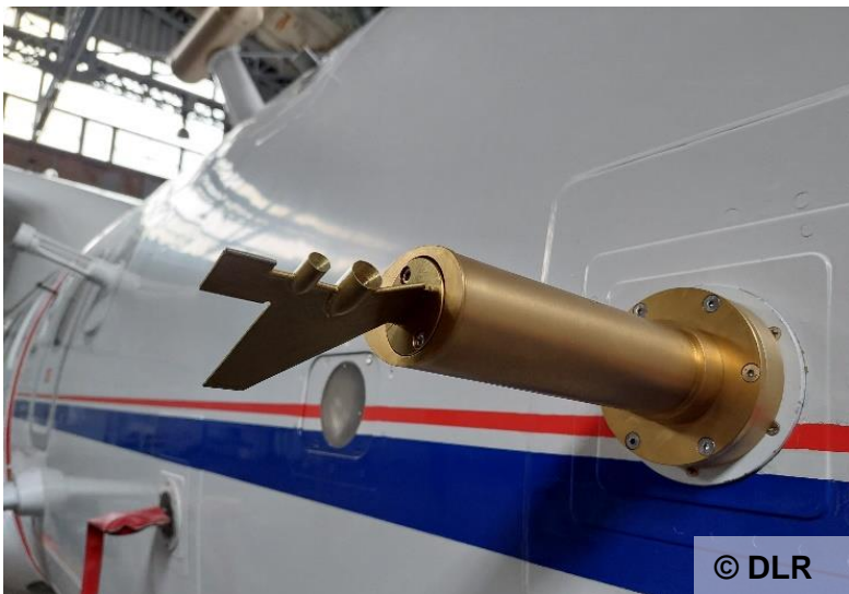
Nevzorov Probe installed on SAFIRE ATR 42
