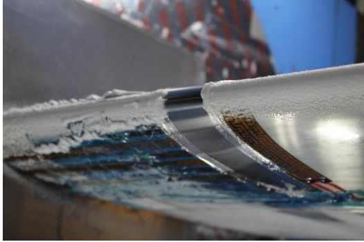
Name: Collins Ice Detection System (IDS) Project partner: Collins Aerospace Copyrights: © Collins
