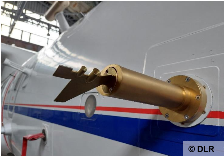
Nevzorov Probe installed on SAFIRE ATR 42
