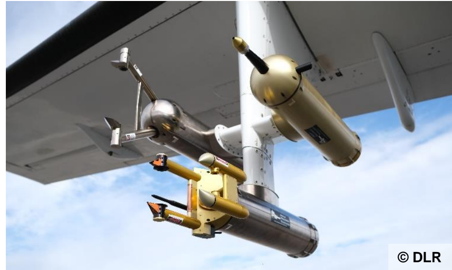
Precipitation Imaging Probe (PIP), Cloud Combination Probe (CCP) and High Speed Imager (HSI) installed on SAFIRE ATR 42
