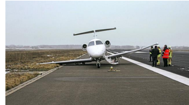
Phenom 100 crash landed due to icing (Source: BFU)
