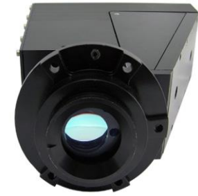
1 st gen. optical sensor direct ptcl. sensing: 2 - 42 \mu\text{m}
