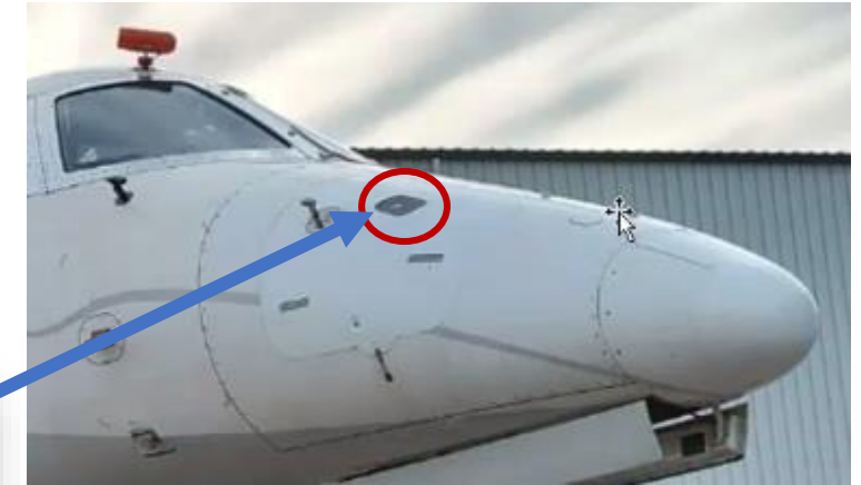
SRP installed on Embraer Phenom 300 © 2023 Embraer
