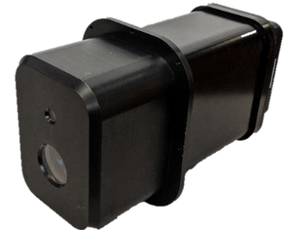
2 nd gen. optical sensor (developed under SENS4ICE) direct ptcl. sensing: 50 - 1000 um background signal sensing: 5 - 50 um
