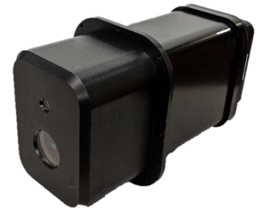
2 nd gen. optical sensor (developed under SENS4ICE) direct ptcl. sensing: 50 - 1000 \mu\text{m} background signal sensing: 5 - 50 \mu\text{m}
