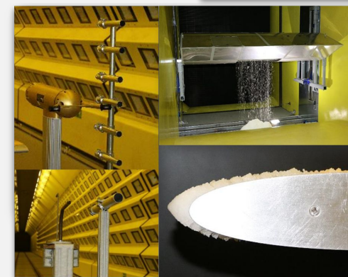
IAG SnowFall snow generation system into RTA Climatic Wind Tunnel and calibration
