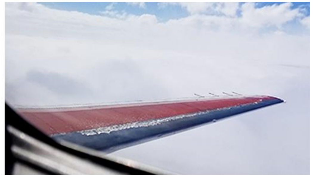
Appendix O icing conditions running back on wing surface of an aircraft.
