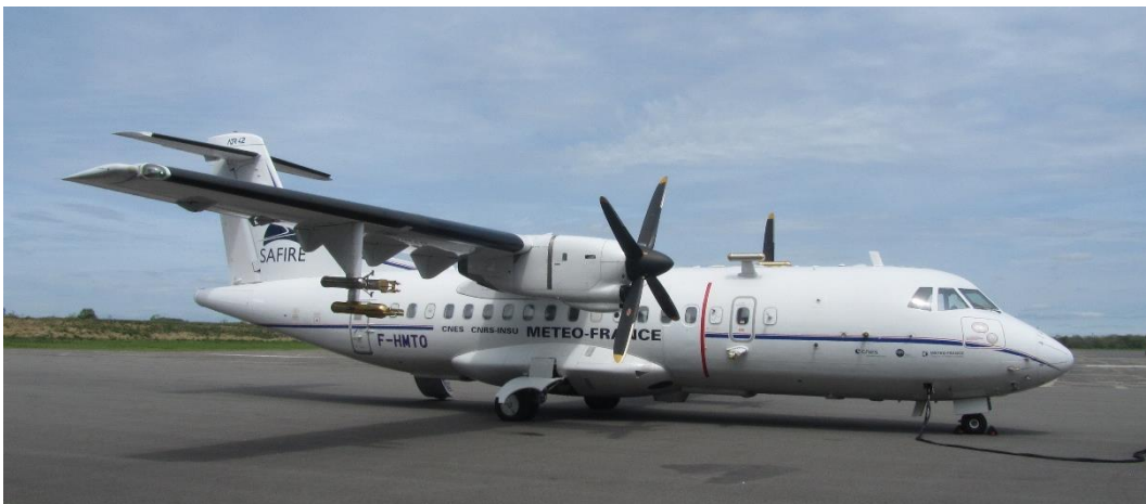
Figure 6: SAFIRE ATR 42 with test sensors and reference instruments [image DLR/ SENS4ICE project].
