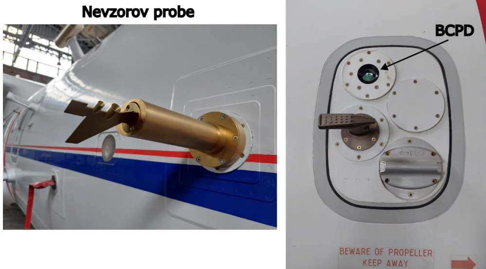
Figure 34: Nevzorov probe and BCPD integrated on the SAFIRE ATR-42 aircraft during the European SENS4ICE campaign [image DLR/ SENS4ICE project].
