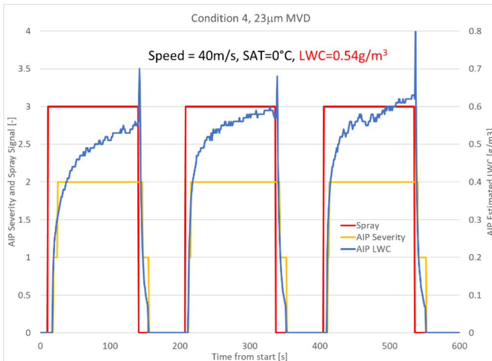
Figure 14: Example of LWC severity detection showing the raw LWC estimate and the associated AIP severity level.
