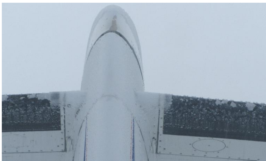
Figure 7: SAFIRE ATR 42 horizontal tail with ice accretion [image DLR/ SENS4ICE project].
