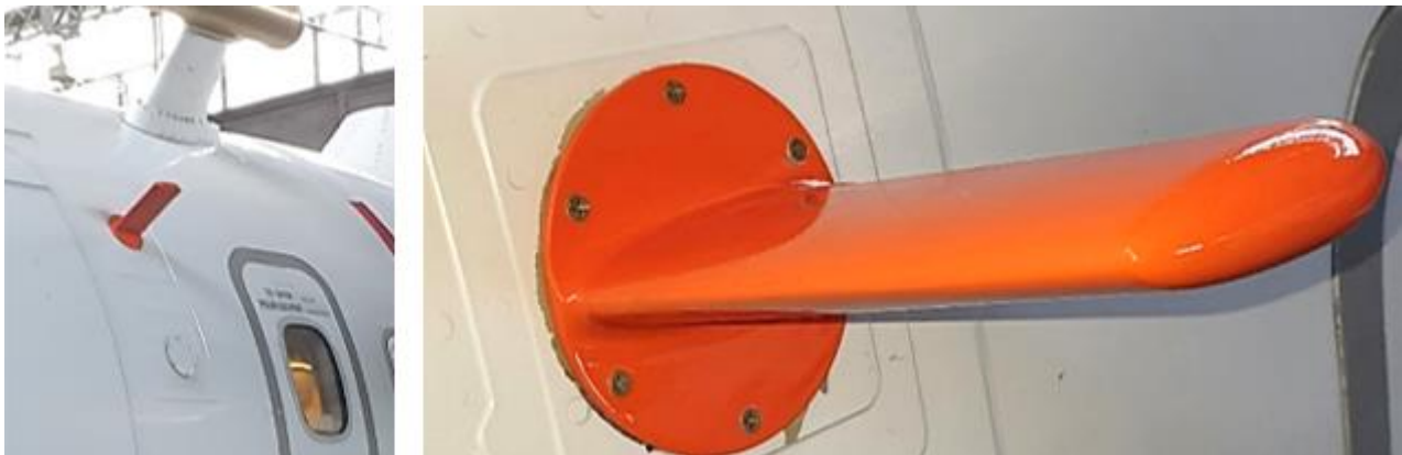
Figure 44: INTA-FOD Flight Test direct sensing probe installed in the left side fuselage of the aircraft [images INTA/ SENS4ICE project].
