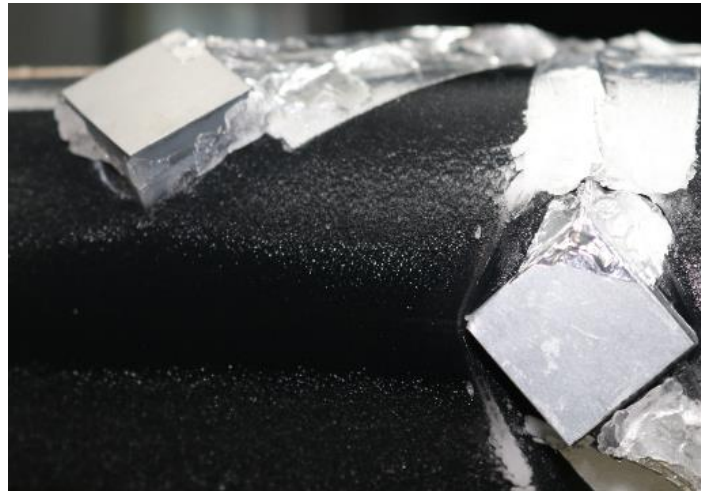
Figure 15: Final icing AIP sensor design being tested in the TUBS BIWT.
