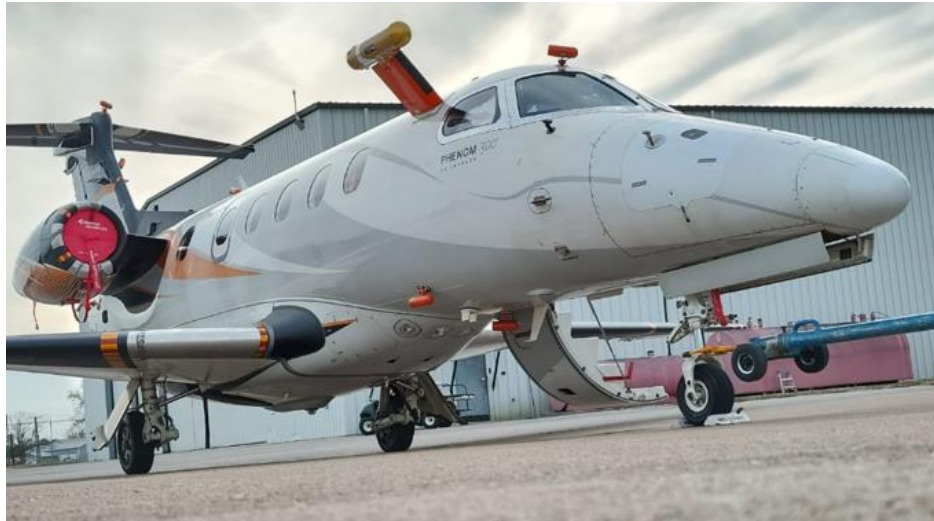
Figure 4: Embraer Phenom 300 prototype with test sensors and reference instruments [image Embraer/ SENS4ICE project].
