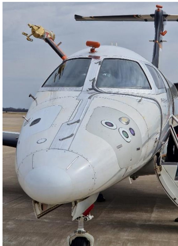
Figure 16: AIP sensors mounted along the centreline of the aircraft [image AeroTex/ SENS4ICE project].
