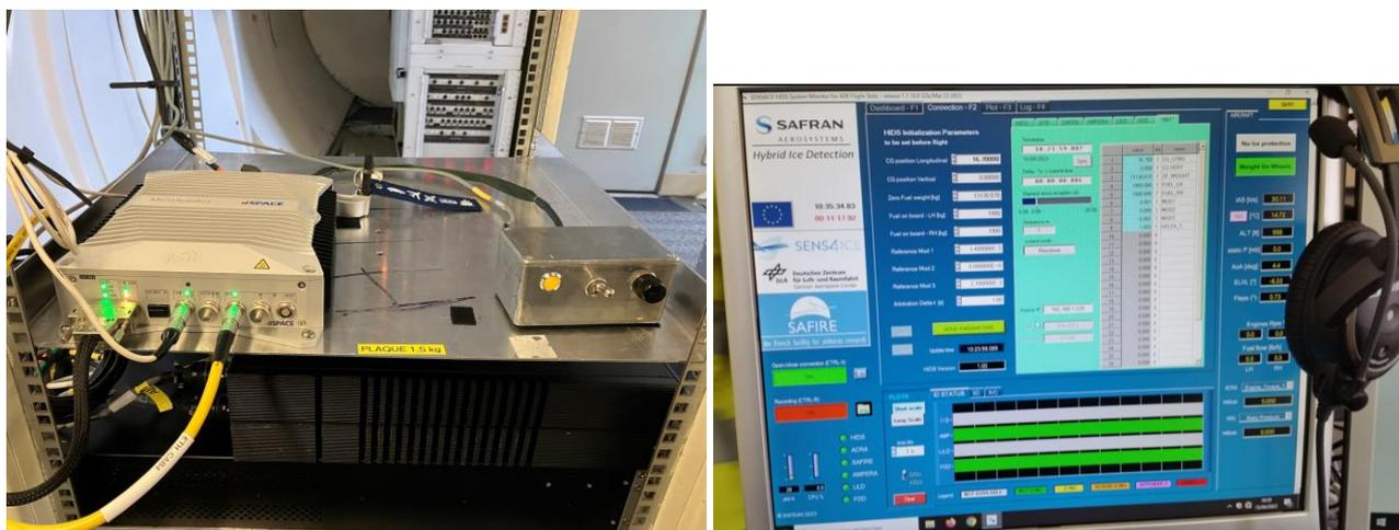
Figure 73: ATR HIDS, on the left, and HIDS-PC user interface, on the right (image credit Safran).
