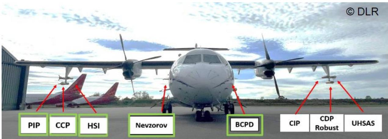
Figure 4: Safire ATR 42 instrumented for European FT campaign (image DLR/ SENS4ICE project)
