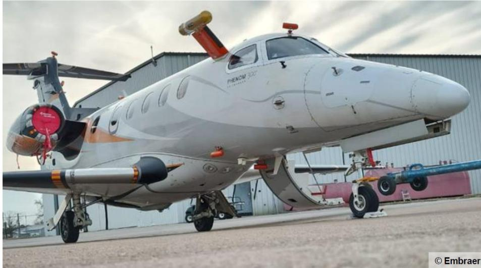
Figure 1: Phenom 300 instrumented for North America FT campaign (image Embraer/ SENS4ICE project).
