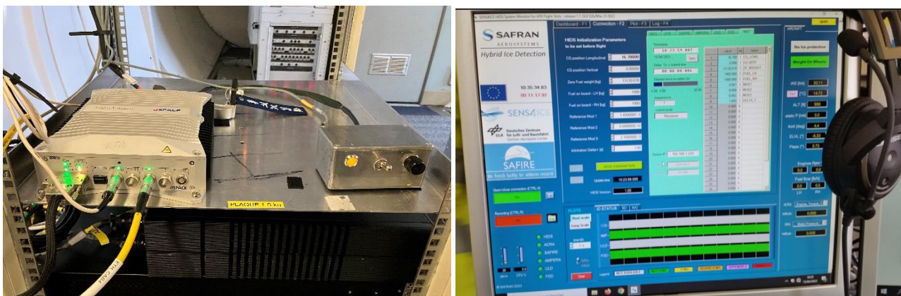
Figure 81: ATR HIDS, on the left, and HIDS-PC user interface, on the right [images SAFRAN/ SENS4ICE project].
