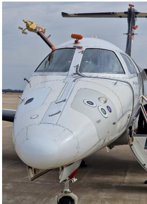
Figure 36: AIP sensors mounted along the centreline of the aircraft [image AeroTex with Embraer permission/ SENS4ICE project].
