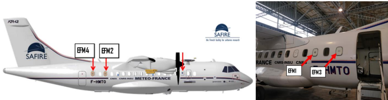
Figure 65: SAFIRE ATR42 aircraft drawing with indication of the two right side windows where the EFM are installed, EFM2 and 4 (left, image Safire). Picture showing the two others mills, EFM1 and 3, installed symmetrically in the left side windows (right, image ONERA/ SENS4ICE project with Safire permission).
