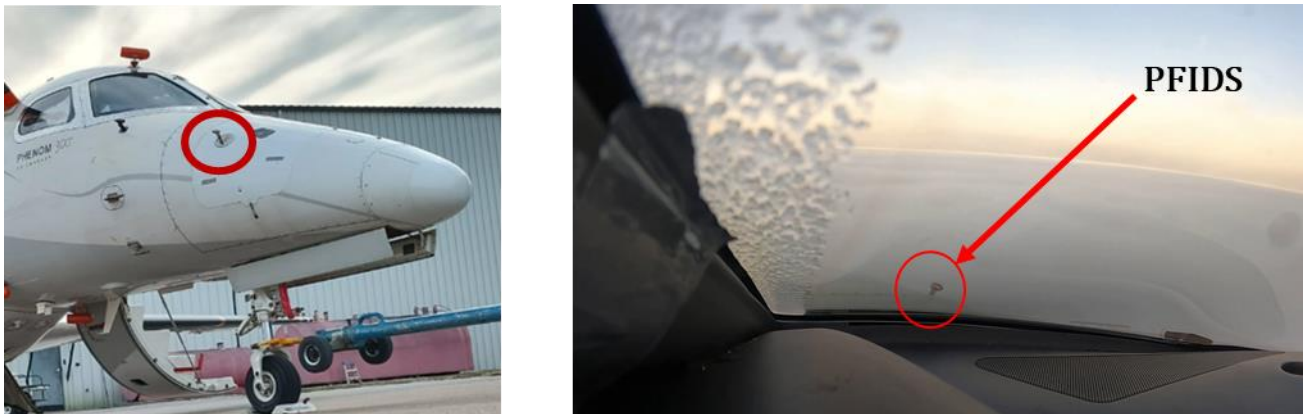
Figure 75: Installation of PFIDS on Phenom 300 [images Embraer/ SENS4ICE project].
