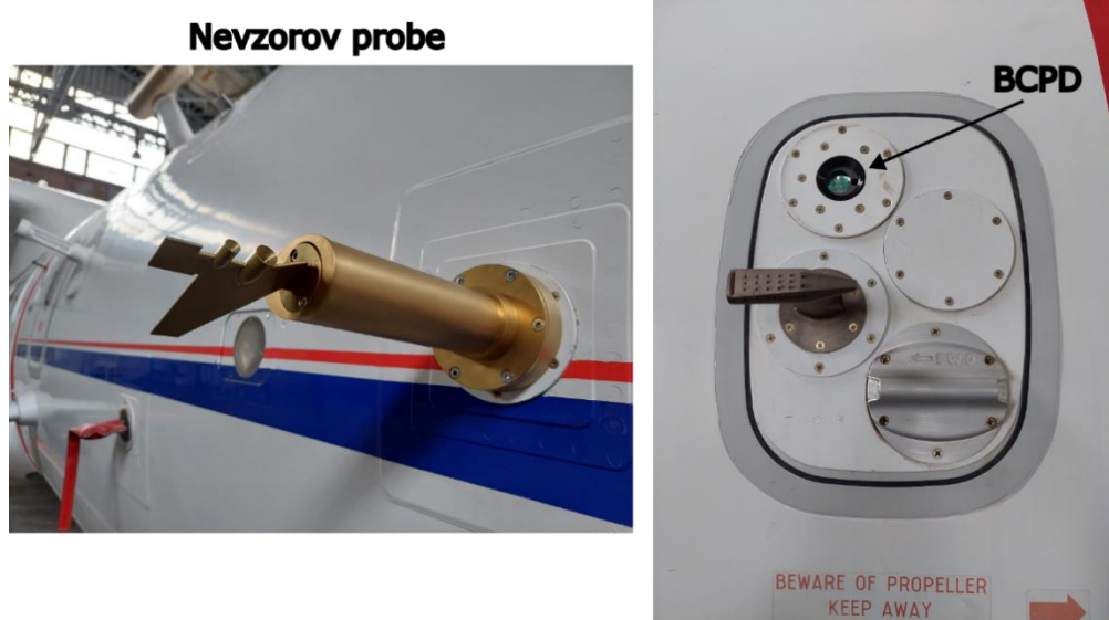
Figure 49: Nevzorov probe and BCPD integrated on the SAFIRE ATR-42 aircraft during the European SENS4ICE campaign [image DLR / SENS4ICE project].
