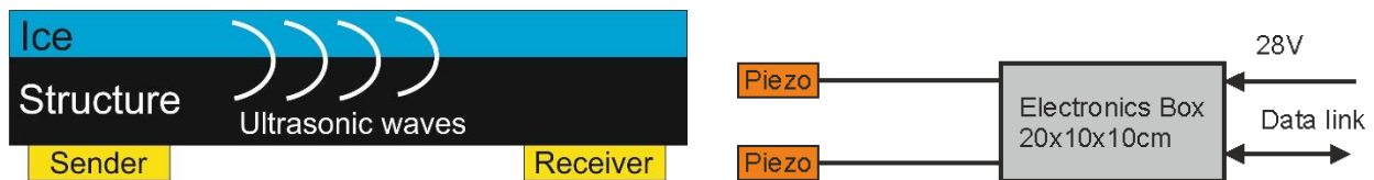
Figure 42: Sensor principle (left) and sensor setup (right).
