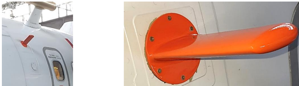
Figure 56: INTA-FOD flight test direct sensing probe installed in the left side fuselage of the aircraft [images INTA/ SENS4ICE project].
